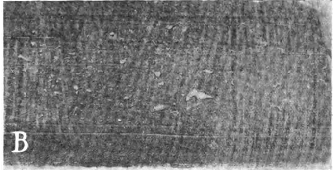
Fig. 1 (B)—34 x 4 Continental tire at 27 pounds pressure per square inch the tread looked good to the naked eye, but in reality was full of small holes
